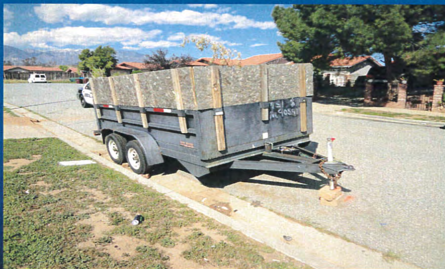
Trailers normally do not have a parking brake and are secured with bricks or rocks
